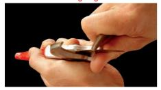
3. Restore the internal chamfer
