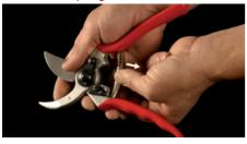
2. Loosen locking segment screw
